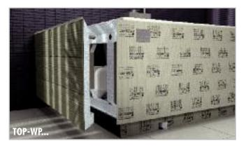
The assembly of this whirlpool surround with footboard and ledge takes place using strong metal fastening pipes, which are fitted into corresponding metal guide sleeves. Therefore, entire front or side sections can be dismantled cleanly and without great effort. Optional light strips are suitable for indirect lighting under the footboard (see page 154).
