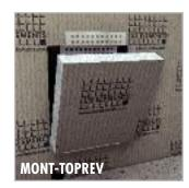
MONT-TOPREV – Easy, fast and flexible. Slip on the MONT-TOPREV (see page 187) retaining section at the top and bottom; press the part previously sawn out of the cladding into the opening against the retaining profile. Seal the joint gap elastically after tiling using silicone.
